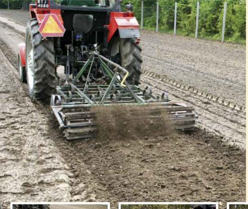
Forest nursery cultivator AUL is designed for cultivating pre-sowed soil thanks to a combination of appliances that enable scarification and leveling of the upper layer of soil, grinding lumps of crusted surface as well as mixing the upper layer and proper pressing for a better capillary rise of water.
