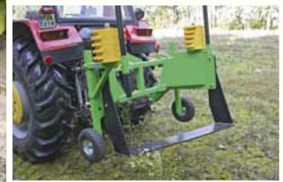
The machine is equipped with weights to assure more stable working, especially while working on a large depth. These should be used depending on the working depth and soil moisture. The operating depth is adjusted using support wheels.
