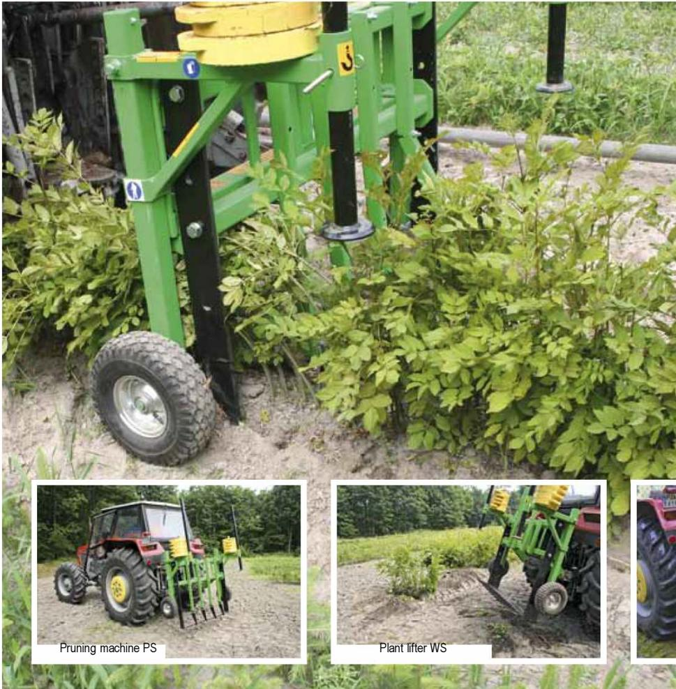
The device is designed for mechanization of tree nursery works. The root pruning machine / plant lifter is mounted on a three-point hitch in tractors working in arboretums. Its simple but solid construction guarantees reliability.
