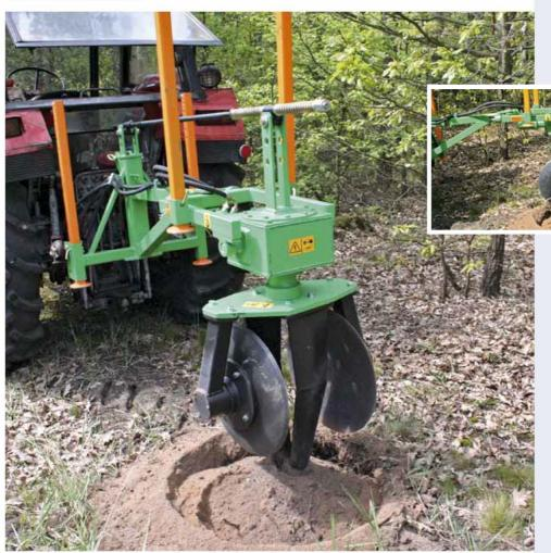
WPG auger has been mainly designed for forestry use. Its small size and weight make the device effective in difficult areas.
