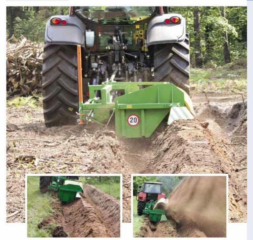
The **ridger** has been designed to form ridges in preparation for planting on temporary wetlands. The rotating head grinds and throws the excavated soil aside of a trapezium shaped trench simultaneously forming a ridge. Trenches prepared by the ridger improve water drainage and planting takes place on the top of the formed ridges.
