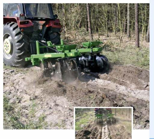
Nizinski's forestry disc harrow has been designed for soil cultivation, loosening and weeding between rows of plants on forest plantations aged 1-5 years. It enables plowing on agricultural areas, initial soil preparation before tillage and preparation of firebreaks.
