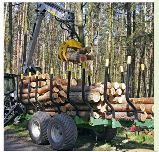
Timber trailers JAR have been designed for forwarding piled and cut to length timber. The trailers are to be used for forwarding timber on distances up to 15 km to timber yards or to hardened surface roads.
