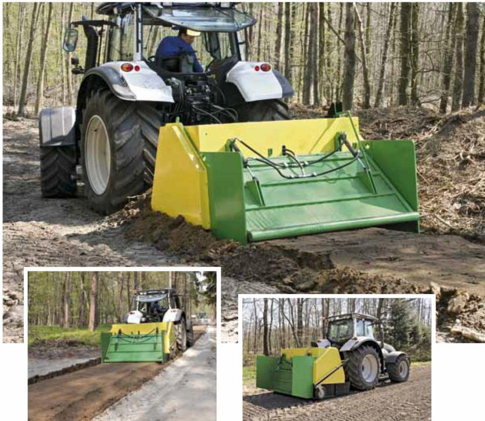
UDM device has been designed for mixing of original material of a dirt road with chemical stabilizers previously applied to the surface. The kind of chemical stabilizer and its depth of mixing must be adjusted to the technology of road rebuild. The machine is mounted on and powered from tractors supplying a minimum power output of 240 HP (a 4 wheel-drive tractor is recommended). Power requirement depends strictly on the applied working depth of the rotor.
