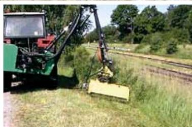
**RBR road shoulder mulcher** has been designed for mowing of roadside and ditches along roads. The device is equipped with a head with a working shaft that is assembled on a hydraulic crane that allows for work in a distance up to 4 meters from tractor's central axis on a slope along the road as well as on a counter-slope.
